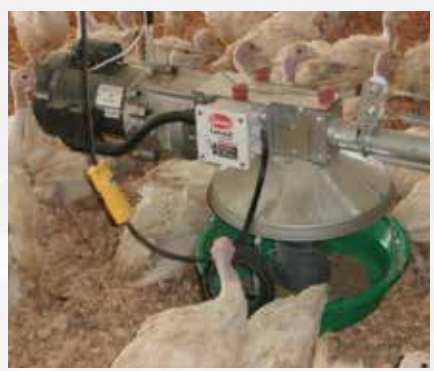
When the feed drops below the infrared sensors, the auger will re-start automatically after a 60 second delay.
