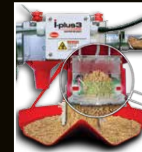
When the feed level breaks all three of the infrared sensors, the auger will stop automatically.
