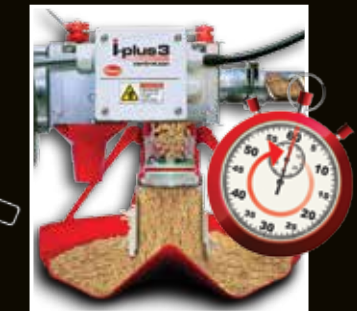
When the feed drops below the infrared sensors, the auger will re-start automatically after a 60 second delay.
