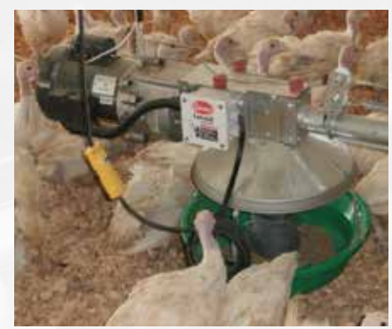
When the feed drops below the infrared sensors, the auger will re-start automatically after a 60 second delay.
