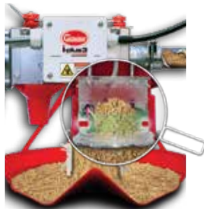
When the feed level breaks all three of the infrared sensors, the auger will stop automatically.
