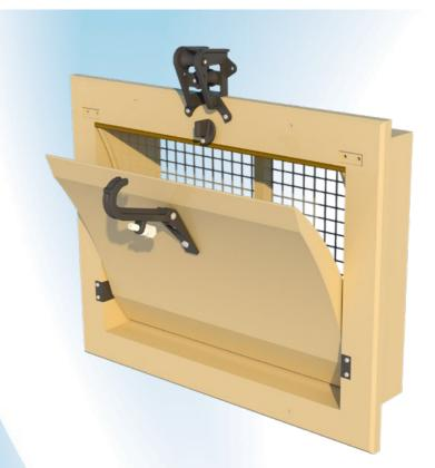
The 1800-VFG-C air inlet valve is made entirely out of high-quality polyurethane. The 1800-VFG-C has a curved inner flap which is hinged in the middle of the house, so when the inner flap opens further then 35% the air also flows underneath the flap. The inlet is controlled by means of a central plastic arm.
